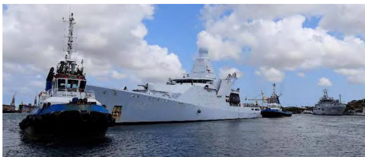
HNLMS Friesland being reversed moored alongside HNLMS Pelikaan by local tugs Manta and Lima II in Willemstad (Curacao), note both heavy fenders alongside HNLMS Pelikaan Photo : Ger Lepel (c)
